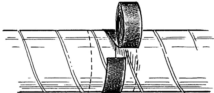
Figure 58. Self-vulcanising sealing tape applied around the duct with overlap.
