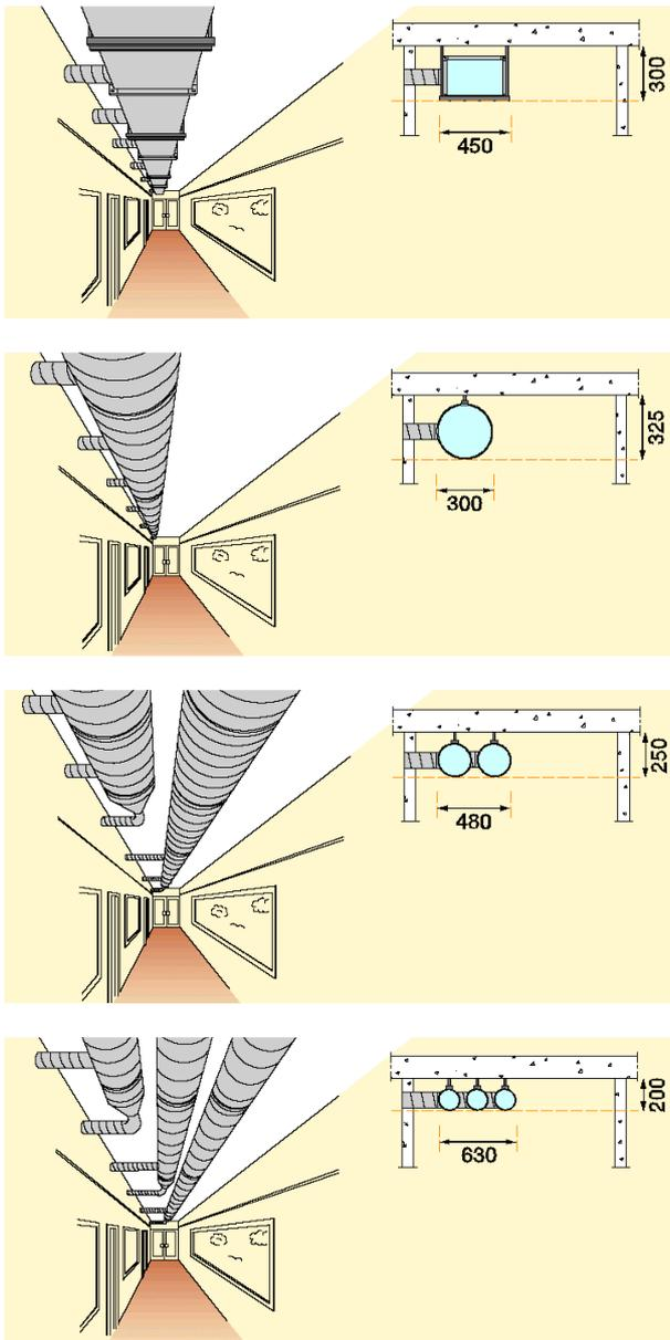
**Figure 67 : Space demand for rectangular or circular duct(s)**
