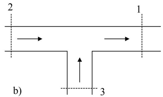
**Figure 44 : Flow in dividing and combining T-junctions.**
