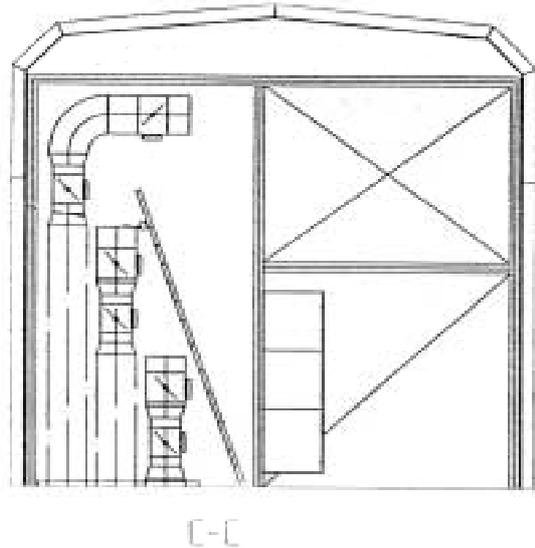
**Figure 104 :** Cross section "C-C" (see Figure 105) through part of the top floor fan room. The (extract) ducts to the left are the ones shown on the photograph (see Figure 103)
