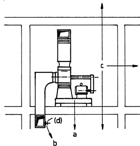
**Figure 54 : The noise from the fan can spread in different ways and directions: Vibrations can result in structure borne noise (a) - Air borne noise carried through the ductwork (b) - Airborne noise in the fan room spreading to adjacent rooms (c), and noise emitted from other ductwork components such as dampers, registers etc (d).**
