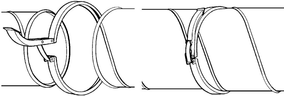
Figure 60. The clips ensure good airtightness and the mechanical stability of the joint. These systems are mainly used for non permanent ductwork or ductwork which has to be cleaned regularly.
