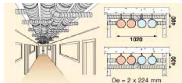
**Figure 76 :** Four possible alternatives starting with rectangular ducts followed by circular ducts.
