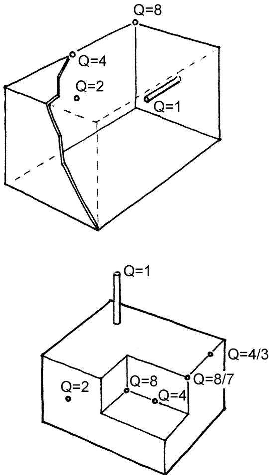
**Figure 56 :** The noise from a source will be influenced by the surrounding surfaces. The directivity factor  $Q$  equals 1 for full sphere and 8 for 1/8 sphere. Near the source each doubling of  $Q$  will result in a 3 dB noise level increase:  $\Delta L = 10 \cdot \log Q$ .
