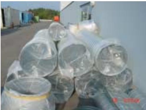
**Figure 51 : Large ducts protected with end covers**
