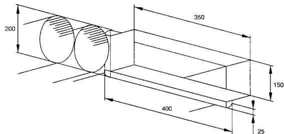
Figure 66 : A flat rectangular duct can often be replaced by several parallel round ducts
