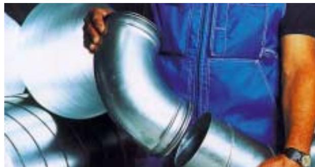
Figure 59. Pre-fitted sealing gaskets for circular ducts. Airtight rivets or plate-screws may be necessary to ensure the mechanical stability of the joint.
