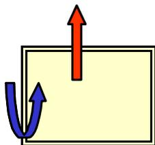
**Figure 1. Schematic representation of a typical natural stack ventilation system. In this figure, the air comes naturally into the building through cracks, slots, trickle ventilators, or other devices, and exits naturally through vertical ducts. The air motion is due to temperature differences or wind or both.**
