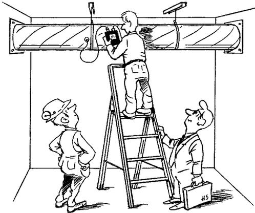
**Figure 82 : Airflow measuring in a duct**
