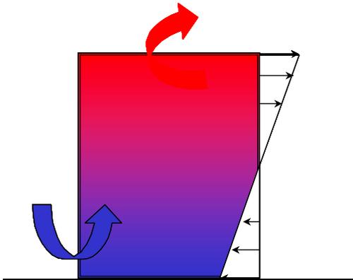
*Figure 22 : The airflow differs between winter and summer due to the stack effect*
