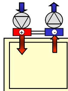
**Figure 3. Schematic representation of balanced SE system. The air is mechanically supplied and extracted through two separate ducted systems. The air handling unit includes a heat recovery unit to transfer the energy of the outgoing air stream to the incoming air stream.**
