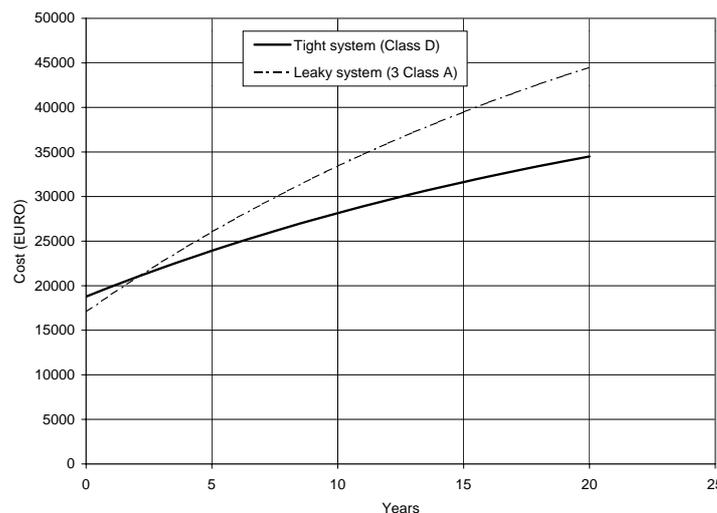
**Figure 32: Comparisons of costs (Net Present Values) of a leaky (3 Class A) and an airtight (Class D) duct system. Calculations are based on the system described in Figure 31 and the parameters shown in Table 3. In that case, the pay-back period is about 2 years.**
