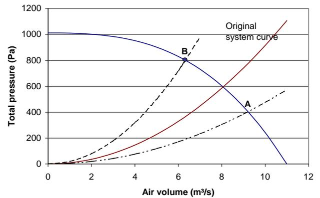
Figure 49 : Illustration of working points for fans
