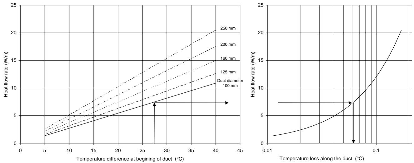
**Figure 24 :** Heat flow rate and temperature loss per unit length of duct for different duct diameters. Airflow rate =  $0.1 \text{ m}^3/\text{s}$ ; 60-mm thick insulation
