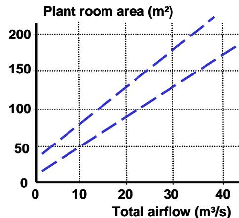
Figure 35 : Estimated plant room area for air handling installations
