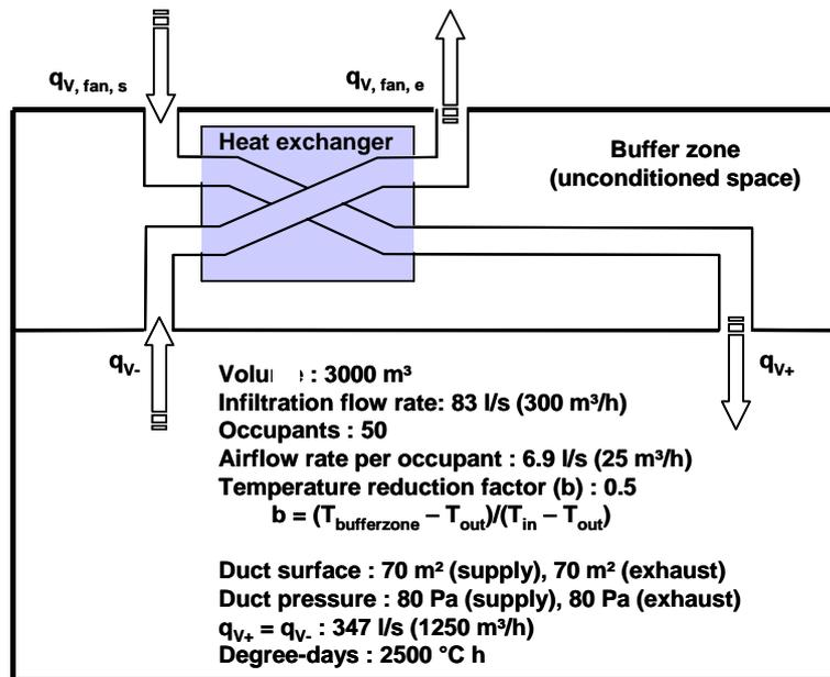
**Figure 31. Schematic diagram of the office building used in the LCC calculations. It is equipped with a balanced ventilation system with heat recovery. The fan airflow rate is adjusted to match the required airflows at the air terminal devices.**
