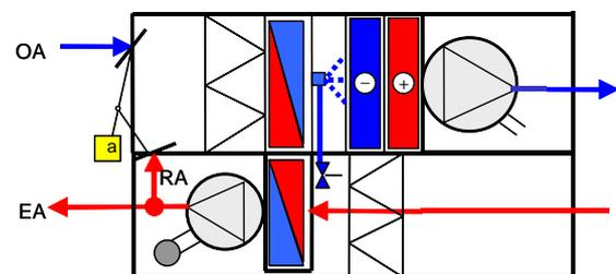
**Figure 52 : To reduce the energy used for heating/cooling the AHU should either be equipped with a heat exchanger or – if the extract air has an acceptable quality – use return air. The shown unit has both possibilities!**
