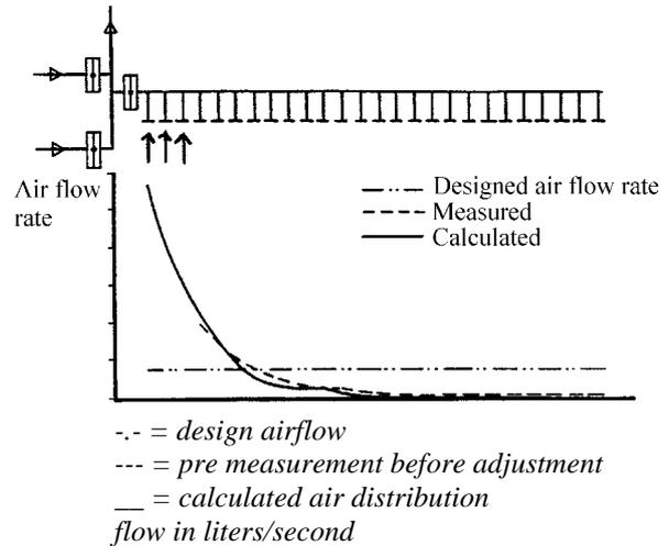
**Figure 84 : Example on calculated and actual airflow distribution on a branch duct with 26 connected extract air registers. Each register comprises an adjustment damper. This example is showing a real installation before reconstruction!**
