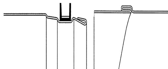
**Figure 73 : Double sealing gasket. Due to larger tolerance range between duct and fitting with increasing duct diameters, the gasket size increases in steps with the duct diameter.**
