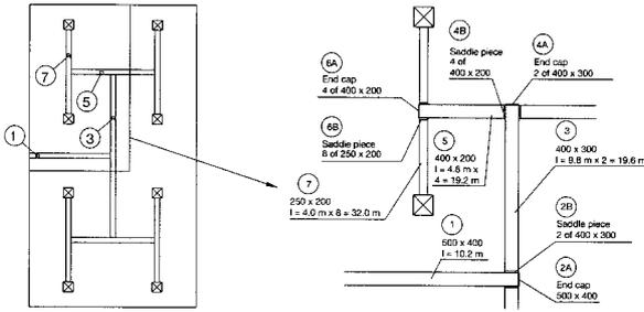
**Figure 36 :** Symmetrical ductwork where the supply air (entering at 1) passes through identical duct components on its way to the registers. The same principle is shown with round ducts in Figure 38.
