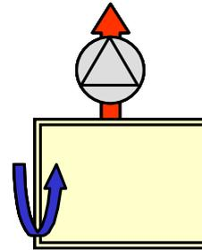
**Figure 2. Schematic representation of E system. The air comes naturally into the building through cracks, slots, trickle ventilators, or other devices, and is mechanically driven out through a central exhaust duct system.**
