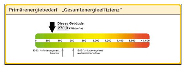
Figure 4: Detail of the Energy Certificate of the Reichstag building, showing the primary energy ranking
