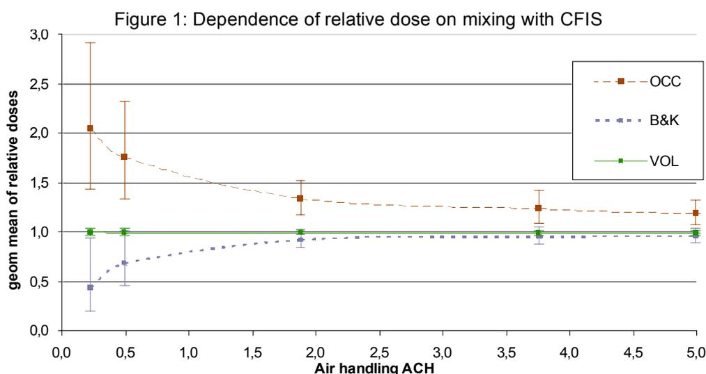
For both CFIS and exhaust cases, increased mixing reduces the difference between means and the variability about the mean. The figures show that increased mixing above a certain rate has little effect on the results. Selection of this “cut-off” rate is fairly arbitrary, but about 0.7 ACH looks reasonable. Comparing the dose curves at equal mixing ACH values, one notices that at equal mixing rates, relative dose
