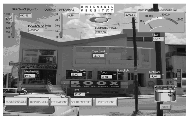
Figure 4: The Georgiadis Building SCADA.
