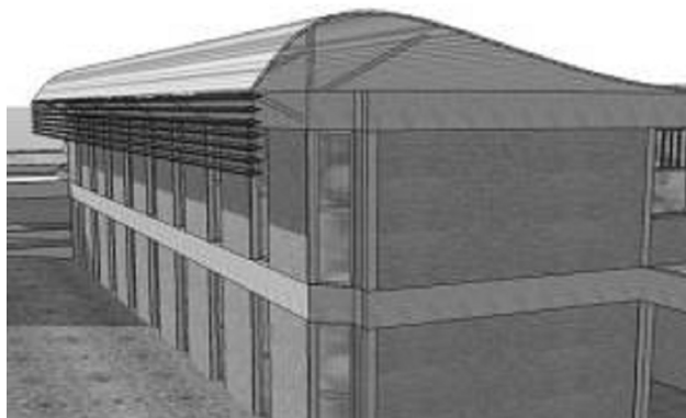
Figure 11: Lightweight cover overlaid to original cover.
