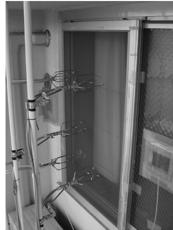
Figure 3: Five Anemometers Setting on Opening
