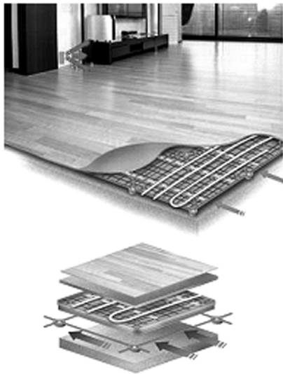
(b) Air flow into the bottom space of the floor heating system Figure 1 : Conceptual diagram for natural ventilation of the raised floor heating system
