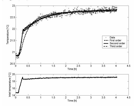
Figure 3: The output of a first order, second order and third order TF model compared with the measured temperature response at sensor position 15
