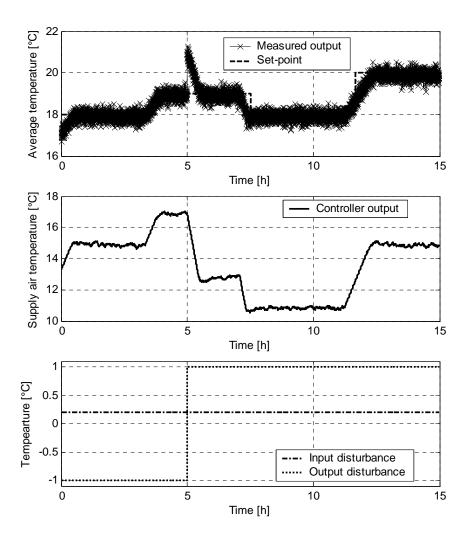
Figure 7: Simulation of the temperature response with measurement noise, input and output disturbances
