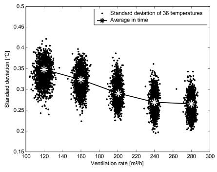
Figure 2: The effect of the ventilation rate on standard deviation of the 36 temperature readings
