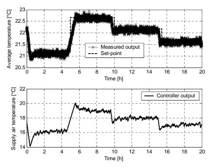
Figure 8: Temperature response as a result of the implemented MBPC
