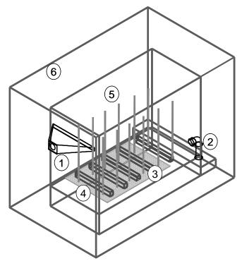
Figure 1: Laboratory test chamber: 1. air inlet, 2. air outlet, 3. aluminium conductor heat sink, 4. shallow hot water reservoir, 5. 3-D sensor grid, 6. envelope chamber or buffer zone
