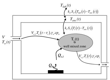
Figure 4: Schematic representation of the WMZ concept.
