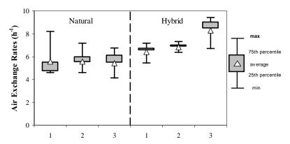
Figure 3: Boxplots of estimated air exchange rates ( $h^{-1}$ ) for natural (single-sided) and hybrid ventilation experiments at  $A_3$  apartment, under calm conditions based on the single-zone (1,2) and multi-zone (3) methodologies
