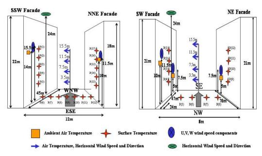
**Figure 1:** A schematic representation of the field measurements performed inside and outside the two urban street canyons (left is Ragavi and right is Ag. Fanouriou canyon)
