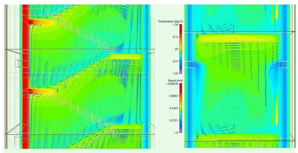
Figure 4:details of fluid flow and temperatures at the first floor (longitudinal and cross section). Case 3 (black-painted) at 04:30h (above) and at 17:00h (below).
