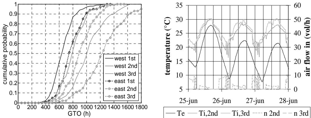
Figure 3: distribution of thermal comfort GTO (left) and comparison of temperatures and flows on the 2<sup>nd</sup> and 3<sup>rd</sup> floor on the east side in the building with mean properties (right)
