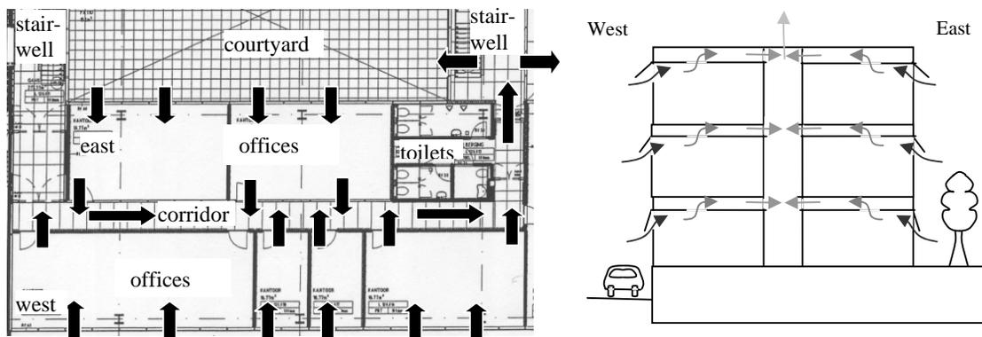
Figure 1: Operation scheme of natural ventilation on a floor plan (left) and on a cross section (right)
