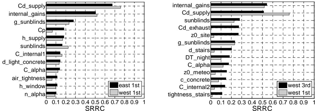
Figure 4: Most influential input parameters on thermal comfort in an office on the west and east side (left) and on the 1<sup>st</sup> and the 3<sup>rd</sup> floor on the west side compared (right)
