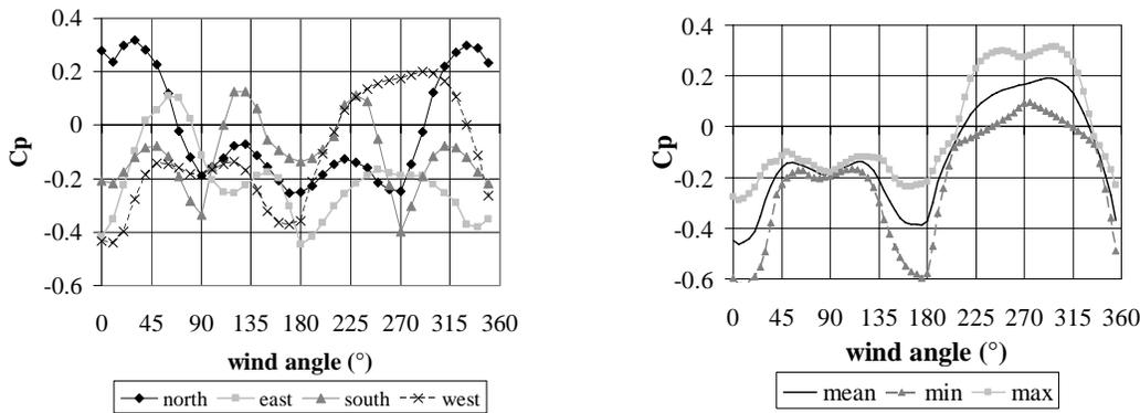
Figure 2: mean wind pressure coefficients  $C_p$  (left) and variation on  $C_p$  on the west side (right)
