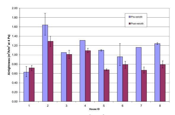
Figure 2. Pre- and post- airtightness measurements in m<sup>3</sup>/h per m<sup>2</sup> of cold walls (except lower floor) at 4 Pa.
