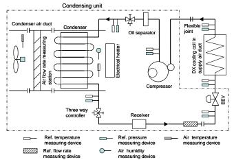
Figure 7: The schematic of the DX refrigerant plant of the experimental station
