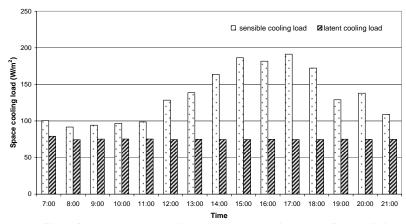
Figure 2: Profiles of hourly space sensible and latent cooling loads for the living/dining room at DOM in the summer design day
