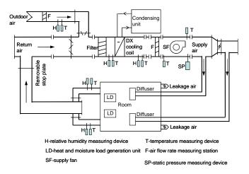
Figure 6: The schematic of the air handling system of the experimental station
