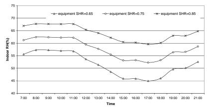
Figure 3: Indoor RH levels at different RAC's equipment SHRs in the living/dining room at DOM in the summer design day
