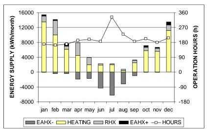
Figure 4: Measured energy supply (Desmedt et al. 2004)
