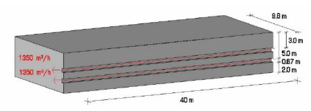
Figure 4: Model geometry and calculation domain (Steeman 2005)
