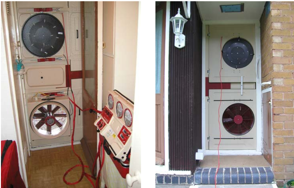
Figure 1: Internal and external view of blower door
