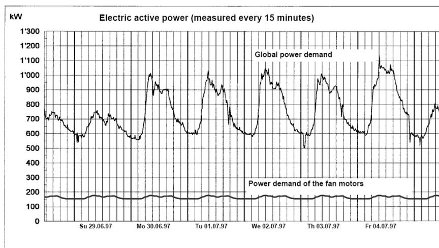
Fig. 3 Measured electricity consumption over a week
