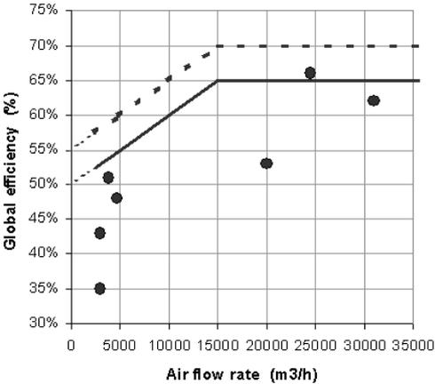
Fig. 2 Comparison of measured efficiency (black dots) and suggested value from Swiss standards
