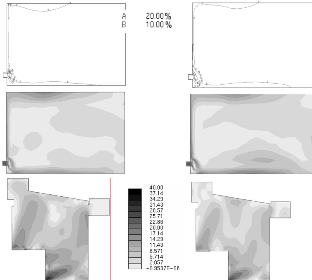
Fig.6 PPD values for variants with Supply Air Convector
