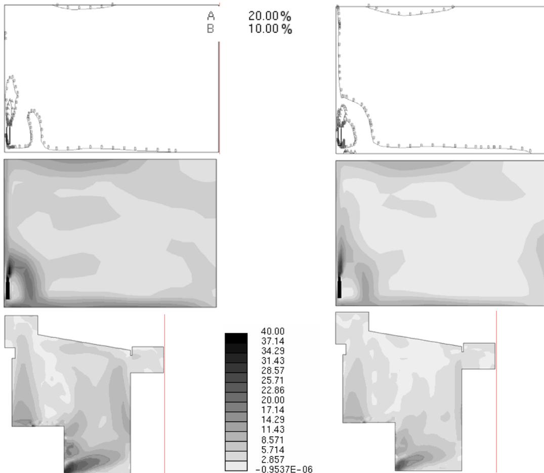
Fig.5 PPD values for variants with Supply Air Radiator
