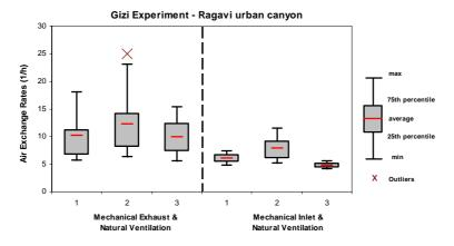
**Figure 9.** Estimated air exchange rates (1/h) for the hybrid ventilation experiments.
