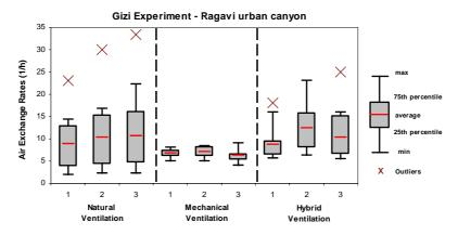
**Figure 8.** Estimated air exchange rates (1/h) for the total number of ventilation experiments.
