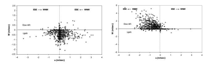
**Figure 7.** Along canyon wind speed, u, against vertical wind speed, w, near a) SSW and b) NNE façade, when the incidence angle of the ambient wind is perpendicular to the canyon axis from southern directions  $(190^{\circ}\pm20^{\circ})$ .
