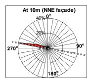
**Figure 5.** Horizontal wind direction outside canyon and near canyon facades, when the ambient wind comes from southern directions  $(190^{\circ}\pm20^{\circ})$ .
