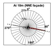
**Figure 6.** Horizontal wind direction outside canyon and near canyon facades, when the ambient wind comes from northern directions  $(10^{\circ}\pm20^{\circ})$ .
