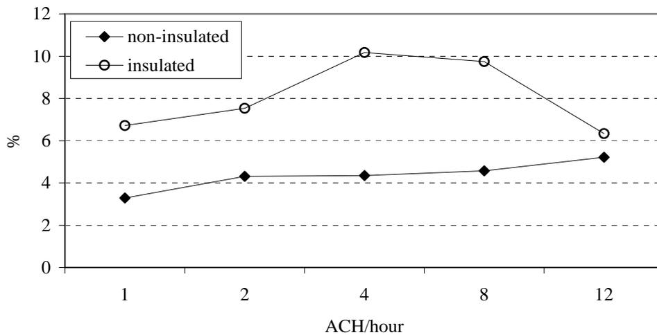
Figure 4: The contribution of the radiative cooling in further reducing the cooling load
