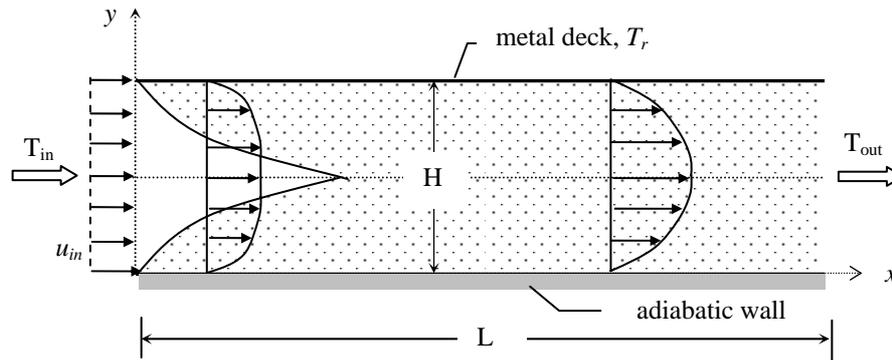
Figure 1: Schematic of the radiative system
