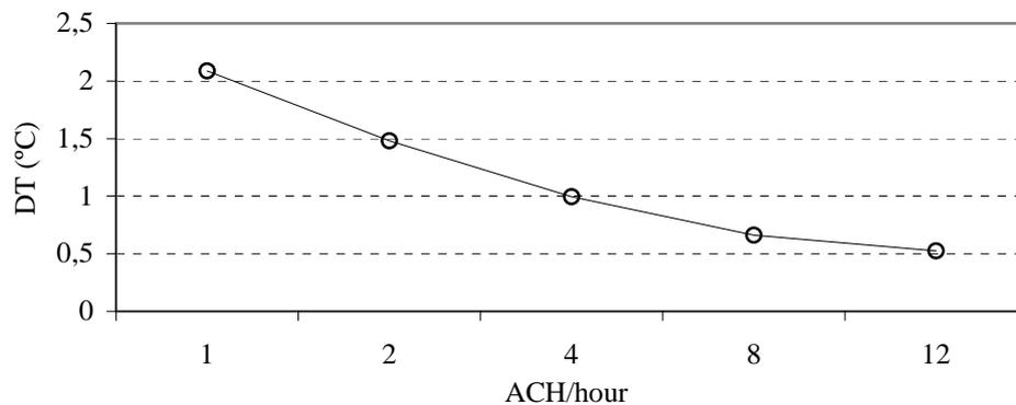
Figure 2: Air flow rate versus DT
