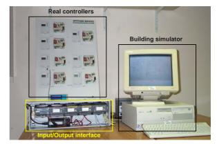
Figure 5: Controller test bench for the QUALISIM project
