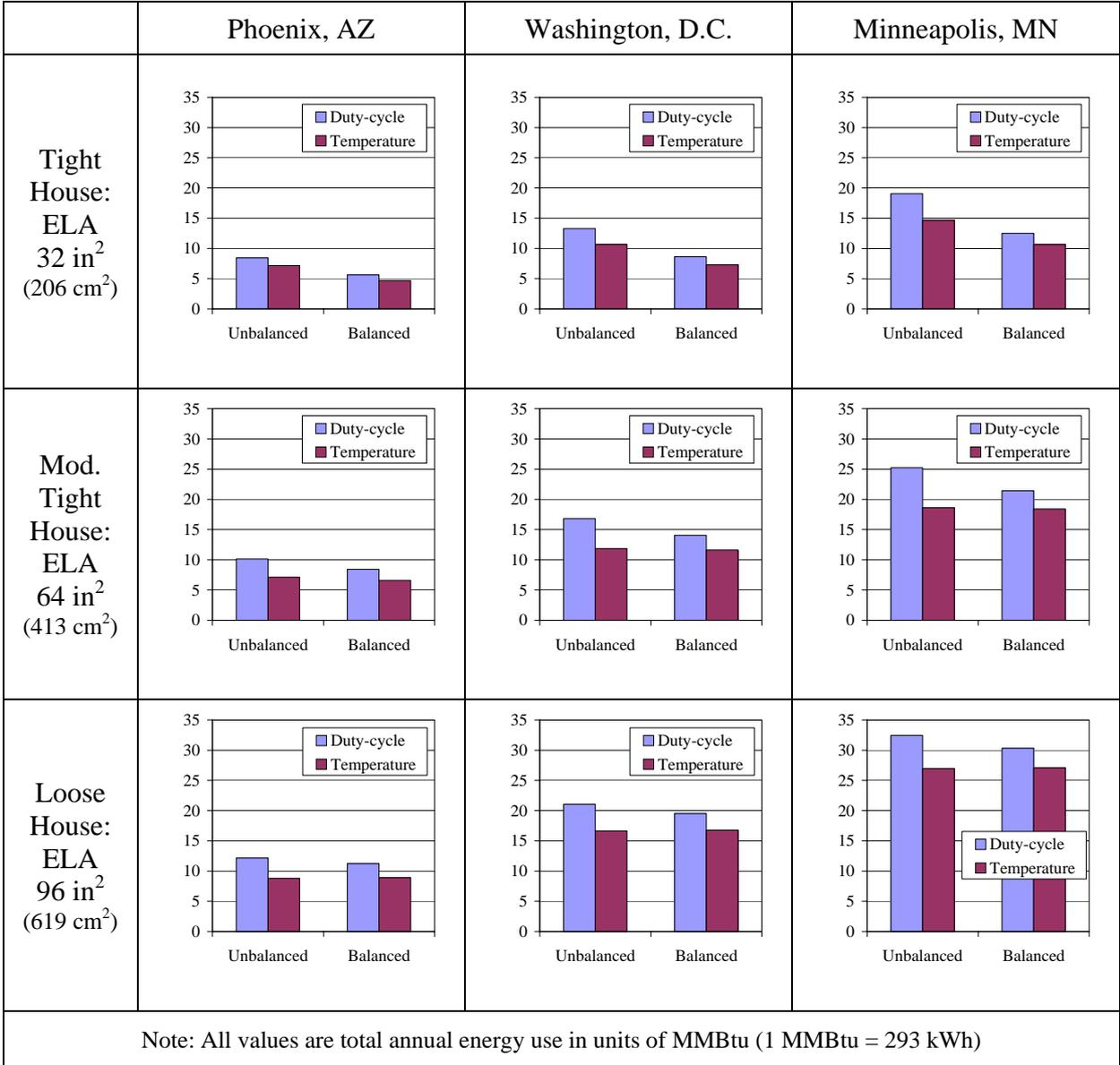
Figure 3. Impact of Effective Leakage Area and System Type on Total Energy Use (Two-story House)
