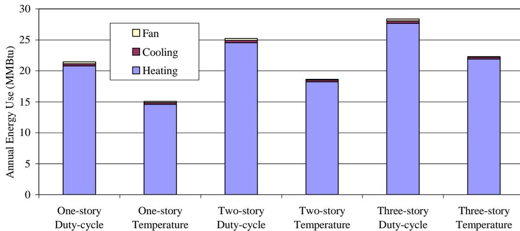
Figure 2. Impact of House Height on Energy Use, Unbalanced System, Minneapolis
