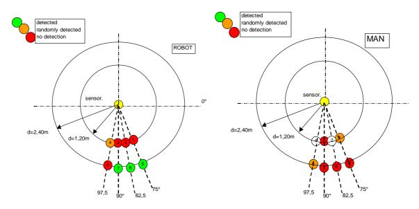
Figure 5 : example of detection by robot on another sensor, and comparison with a detection with man movement
