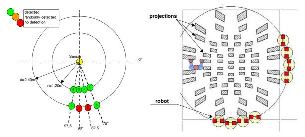
Figure 4 : example of detection from robot compared to the faces projection given by the manufacturer
