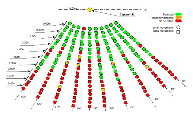
Figure 6: complete detection on a sensor
