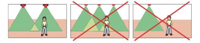
Figure 1 : correct position of infrared sensors in the room
