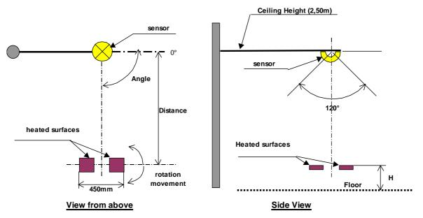
Figure 2 : description of the test installation
