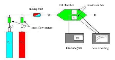
For 3 to 6 values of CO2 concentrations are determined, according to the range of each sensor (even more if the range of measure of the device is widened) and they are injected in the test chamber. Considering the weak volume of the test chamber the completion of this one is considered as immediate.
