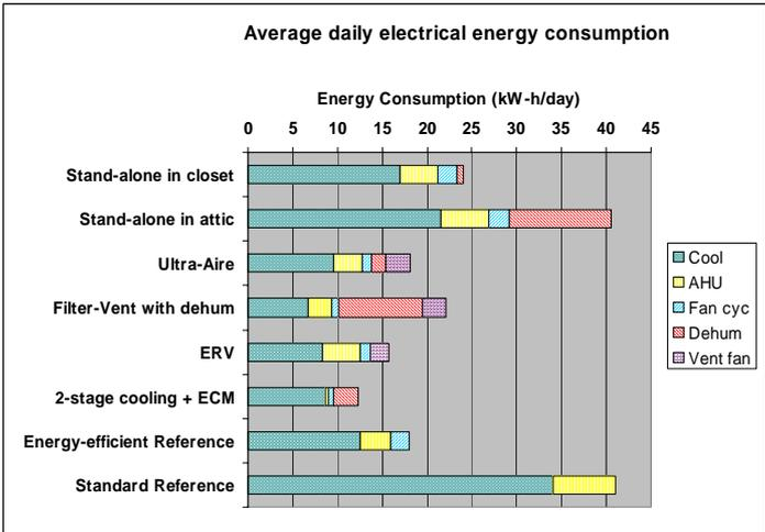
Figure 2: Average daily electrical energy consumption for all mechanical equipment monitored
