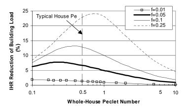
Figure 2. Reduction of building load using equal participations. The typical house Pe is for the case where one third of the building load is due to infiltration with no heat recovery.
