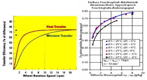
Figure 1: Effectiveness of recovery heat exchangers (Harriman et al., (2001). Furter and Keller, (2000).)
