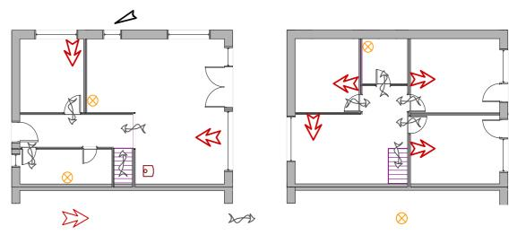
Figure 6: Floor plan with position of stove and air distribution of the simulated two-storey dwelling
