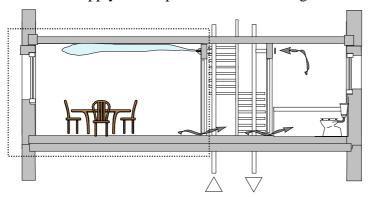
Figure 3: Typical Passive House ventilation configuration with far throw jet air inlet positioned at the internal wall to the corridor. The space covered by measurements is indicated by dotted lines
