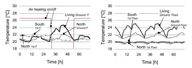
Figure 7: Room air temperatures with internal doors open. Stove fired twice a day (morning and evening) during one specific day; air heating the days before and afterward (left).
