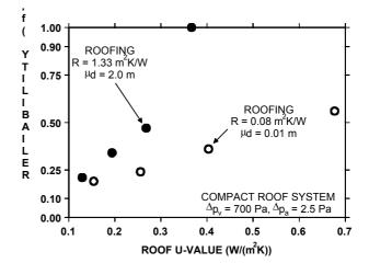
FIGURE 5: Effect of diffusion thickness of vapour retarder on condensation amounts at underlay surface
