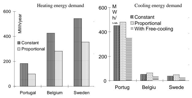
**Figure 5:** Heating and cooling energy demand of the large office building as a function of the control strategy, for different virtual locations.
