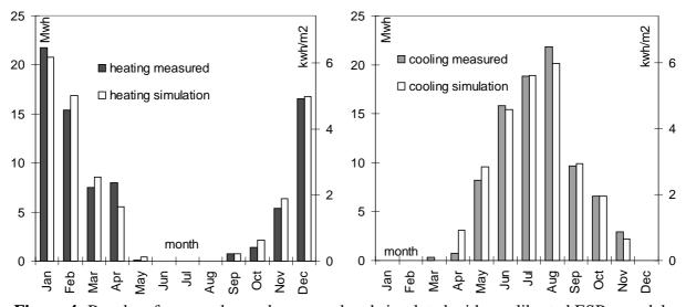
Figure 4: Results of energy demand measured and simulated with a calibrated ESP-r model
