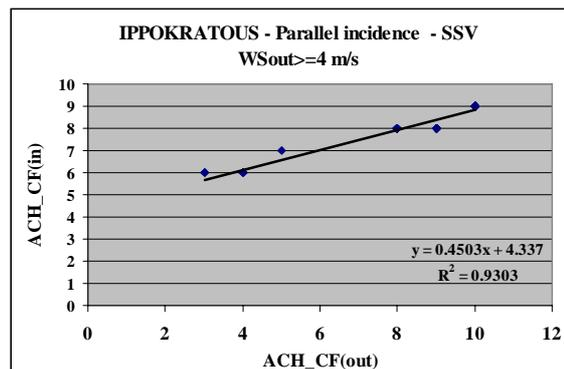
Figure 6. Parallel incidence – Single Sided Ventilation ( $WS_{out} \geq 4m/s$ )
