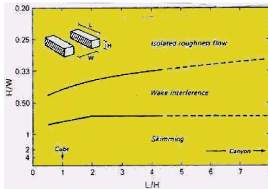
Figure 3. Threshold lines dividing flow into three regimes as functions of the building ( $L/H$ ) and canyon ( $H/W$ ) geometry
