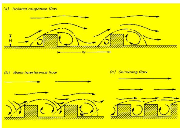
Figure 2. The flow regime associated with air flow over building arrays of increasing  $H/W$
