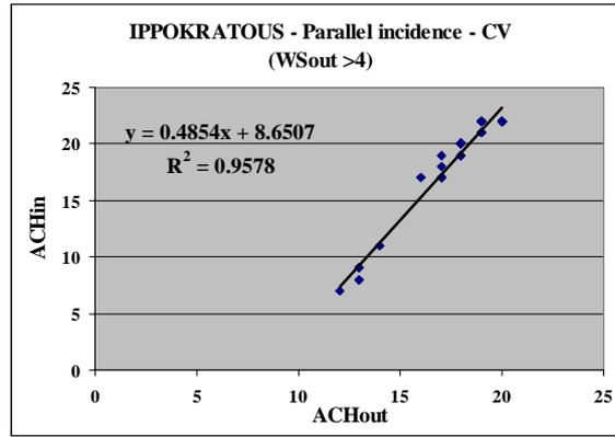
Figure 7. Parallel incidence – Cross Ventilation ( $WS_{out} \geq 4m/s$ )
