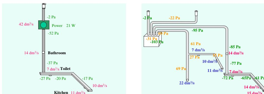
Figure 1 Measurement results of an exhaust only and a balanced system.
