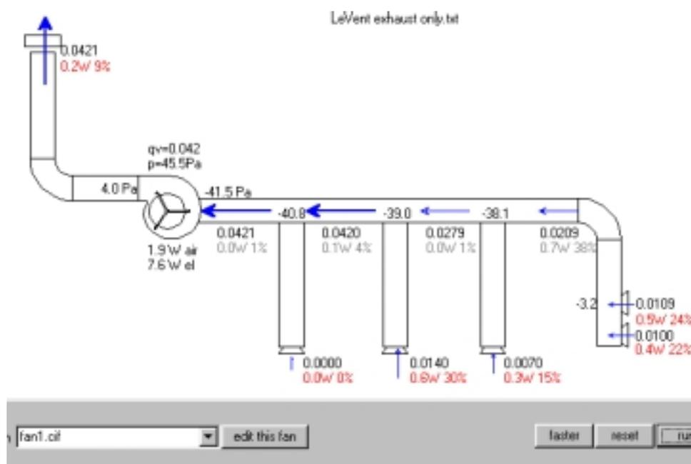
**Figure 3** Scheme of the TipVent duct program
