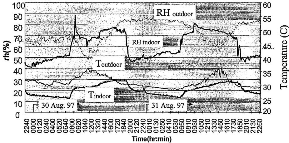
Figure 2. Monitored RH and temperature on the 1st and 2nd day
