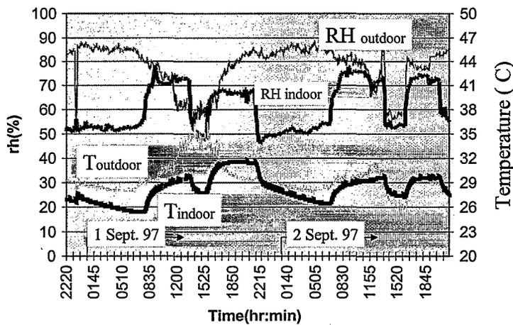
Figure 3. Monitored indoor and outdoor RH and temperature on the 3rd and 4th days
