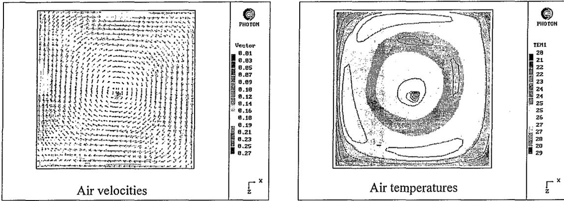
Figure 3. Plan view showing air velocities and temperature contours 1.8m above floor level
