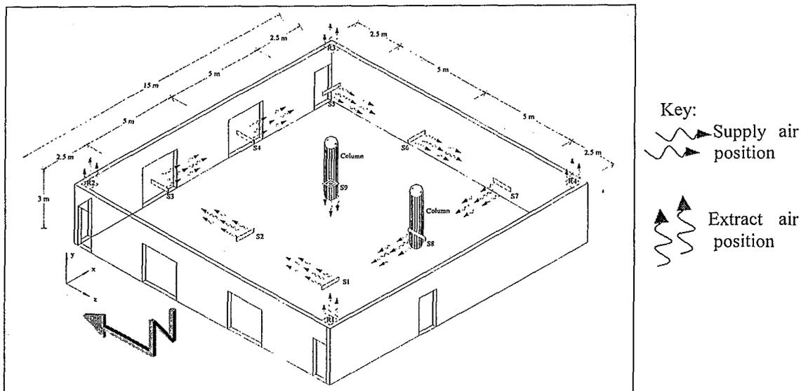
Figure 2. Air distribution layout used in the simulation.
