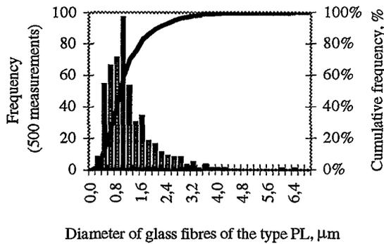
Figure 2. The distribution of cumulative frequency and frequency of occurrence of the given diameter of glass fibres - type PL.
