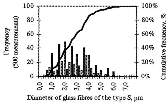
Figure 3. The distribution of cumulative frequency and frequency of occurrence of the given diameter of glass fibres - type S.
