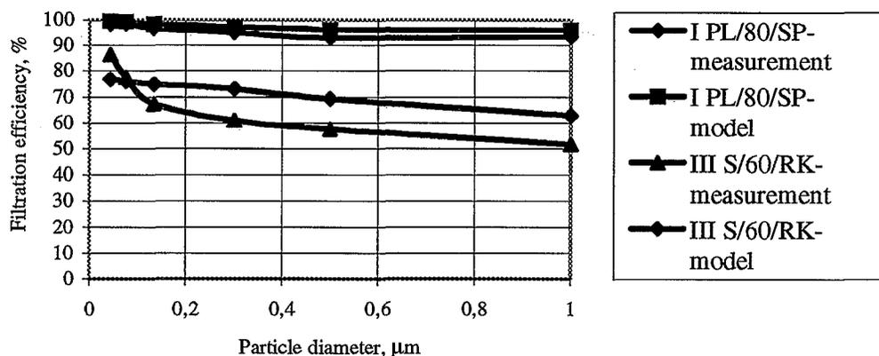
Figure 1. The comparison of the characteristic of the filter obtained on the basis of the proposed model of the filtration process and real for the non-wovens I PL/80/SP and III S/60/RK.
