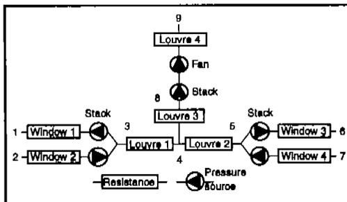
Figure 3. The ventilation model
