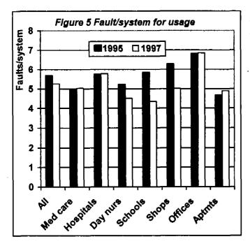
The number of faults FA+FF in general was 5.3 faults/system for 1997 compared to 5.7 faults/system for 1995. If a system is not approved it has in general more than 3 faults that each cause a disapproval of the system, see figure 5.
