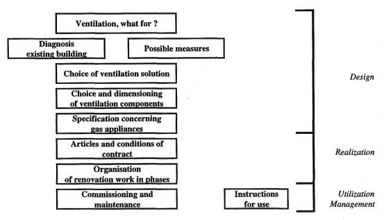
Figure 1: different stages in renovation work
