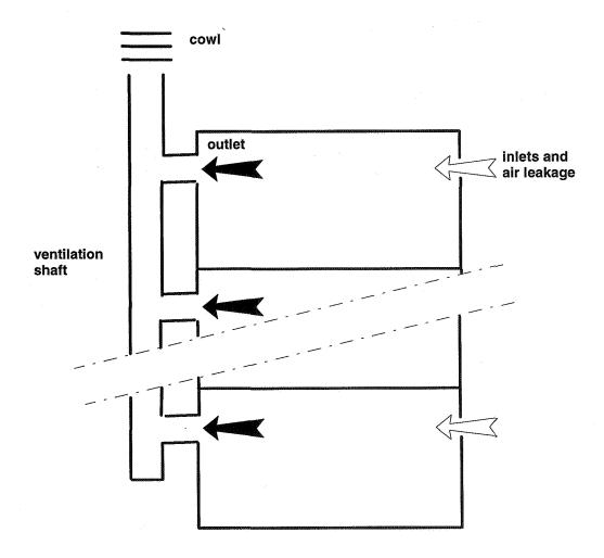
It takes into account the combined effects of driving forces such as wind-induced pressures, thermal buoyancy and mechanical forces due to motorised cowls.
