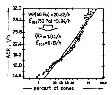
Fig. 3. Normal distribution of air change rate for 104 zones located in one of the tested buildings (results of pressurization tests at Δp about 50 Pa - before termorenovation)
