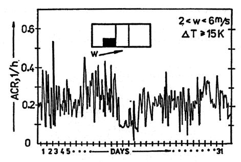
Fig. 4. Variability of air change rate in a room on the fifth floor of one of the tested buildings after its thermorenovation (measurement results employing the method of constant SF<sub>6</sub> emission)
