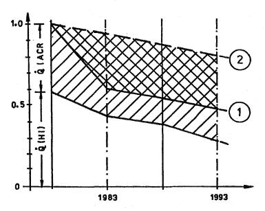
Fig. 6. Changes of ventilation heat demands in the balance of basic heat losses (1983, 1993 - years when new standards were introduced)
