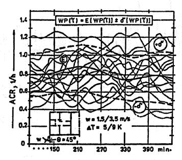
Fig.2. Variability of air change rate in a flat on the third floor of the tested building (measuremement results employing the method of NO<sub>2</sub> constant concentration and concentration and covering 14 four-hour period before thermorenovation)
