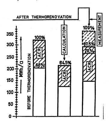
Fig5. Comparision of heat amounts used to heat 9 identical multifamily buildings (calculations were made by means of TRYNSYS and SYMWENT)
