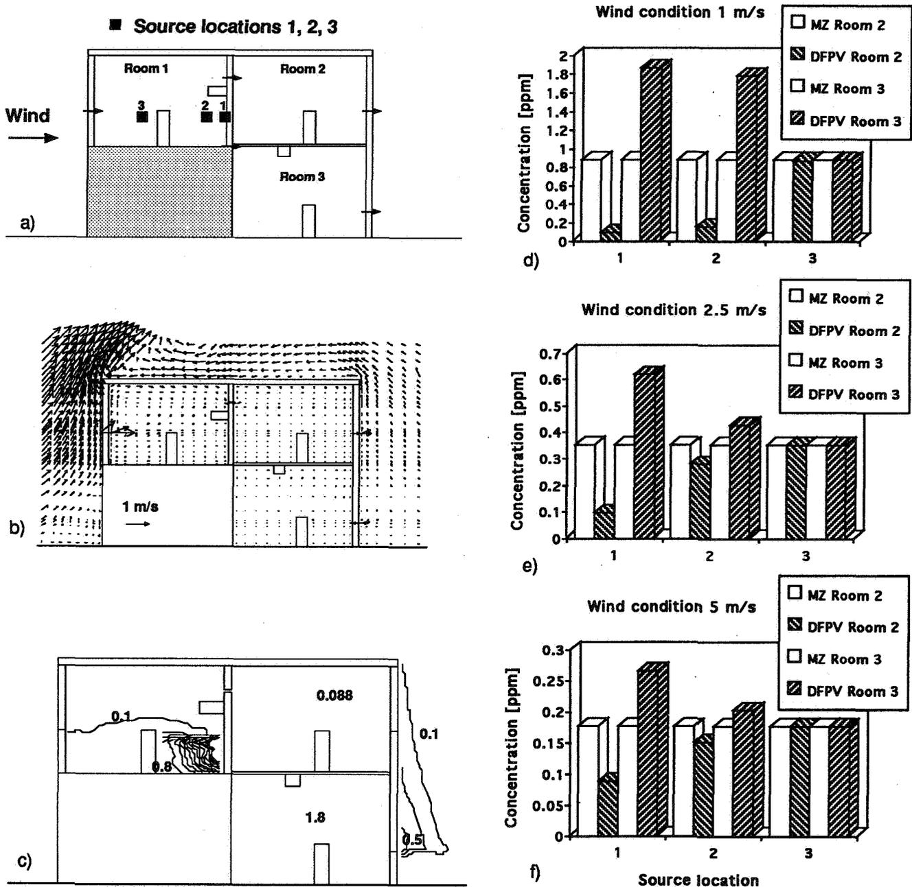
Figure 3: a) Sketch of the geometry with 3 rooms. b) Air flow field and c) contaminant contour lines for Case 1.1. d-f) Multizone and DFPV values in Room 2 and Room 3 for the 3 cases with wind velocities 1, 2.5 and 5 m/s.
