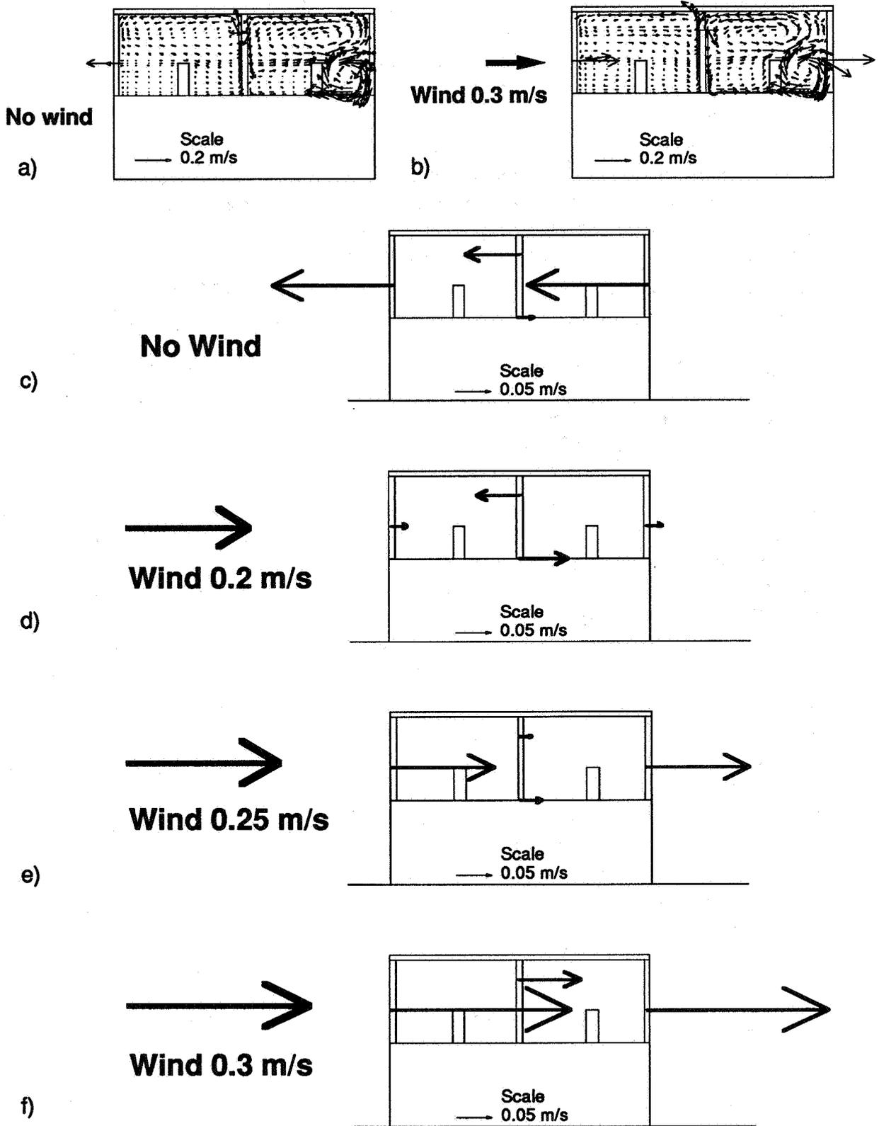
**Figure 4:** Case with 2 rooms and 4 cracks: a) Air flow pattern without wind. b) Air flow pattern for wind velocity 0.3 m/s. c-f) Air flow in cracks for wind velocities 0.0, 0.2, 0.25, 0.3 m/s.
