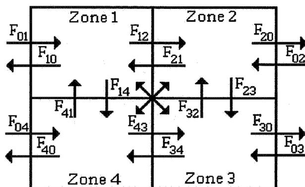
Figure 5 - Schematic diagram of the four zone model.
