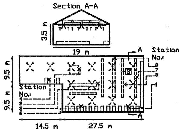
Fig 1. Layout and cross-section of the plant designed for MIXVENT (not to scale)
