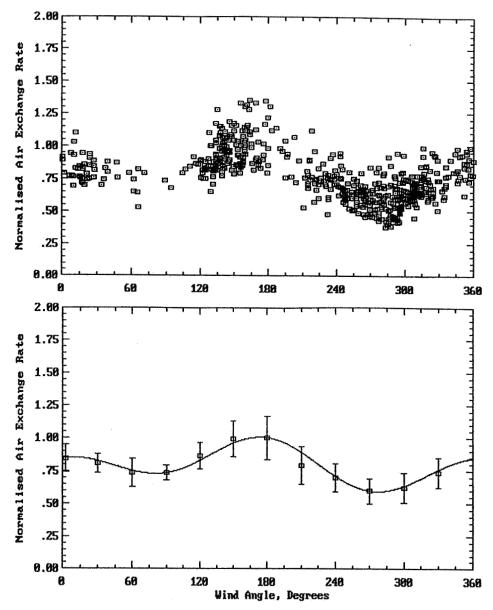
Figure 4. Measured wind shelter for House #4 with 0.075 m restriction orifice in 0.15 m I.D. flue (580 hours)
