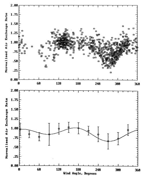
Figure 2. Measured wind shelter for House #5 with no flue (823 hours)
