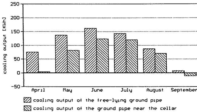
**Fig. 7 Cooling output of the ground heat exchanger**
