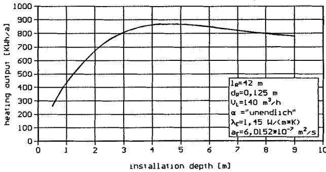
**Fig. 11 Heating output of the ground heat exchanger**
