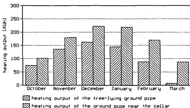
**Fig. 10 Heating output of the ground heat exchanger**
