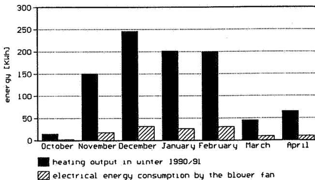
**Fig. 9 Heating output of the ground heat exchanger**
