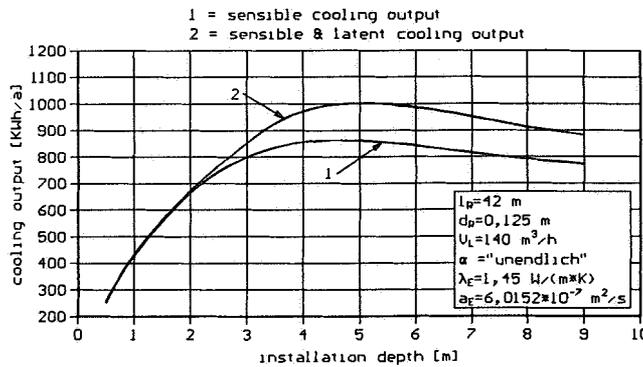
**Fig. 12 Cooling output of the ground heat exchanger**
