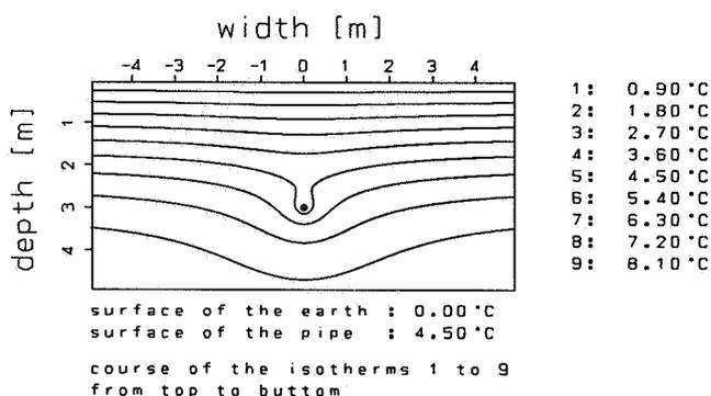
**Fig. 2 Earth temperature field** employed. The volume flow was 140 m<sup>3</sup>/h. Inspection of the temperature field near to the ground pipe and consideration of the fact that, according to Ottel /11/,
