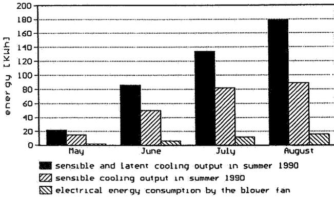
**Fig. 6 Cooling output of the ground heat exchanger**
