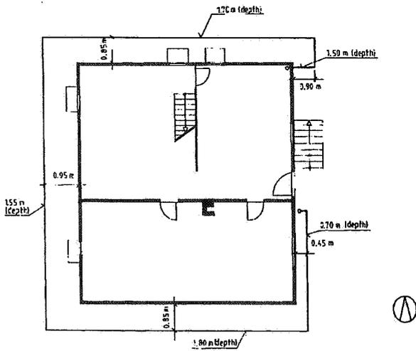
Fig. 4 Scheme of the ground heat exchanger
