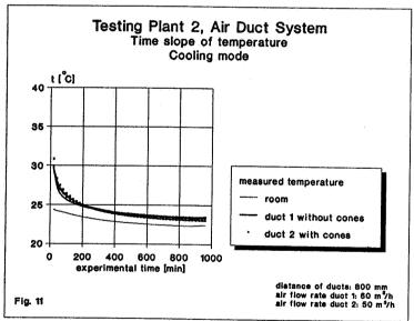
The investigation showed that the pressure drop of the duct equipped with cones is much to high for practical applications. For this reasons this construction is not further considered.
