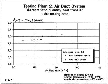
The coefficient of heat transmission related to the air flow rate is shown in Fig. 6 and the characteristic quantity heat transfer in Fig. 7. These two figures are compared directly, because the distance of the ducts is the same as the width of the testing area (800 mm). Only for a distance lower than 500 mm the characteristic quantity is depending on the distance of
