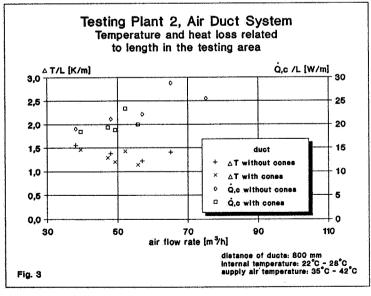
It is evident that for both systems the temperature difference decreases slightly, whereas the convective heat loss rises strongly with increasing air flow rate. Considering an air flow rate of 50 m<sup>3</sup>/h the temperature difference of plant 1 is 2K, of plant 2 only 1,3K.
