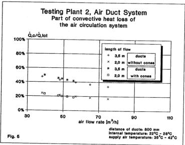
Fig. 4 and 5 show the part of convective heat loss of the air circulation system related to the air flow rate. For an air flow rate like in practice of 40 m<sup>3</sup>/h the part of the surface heating in the testing plant 2 is 40%, whereas in plant 1 it's greater than 70% because of the great storing capacity of the floor. This effects low temperatures at the air inlet so that
