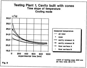
The influence of the thermal inertia of the cavity floor construction for the heating respectively the cooling mode is recognizable in Fig. 8 and 9. Only after 10h working time the storage process in the floor was finished and the difference between the temperature at the air inlet and the room temperature is too low. Fig. 10 and 11 show a lower thermal inertia because the storing capacity is not so high. At the air inlet of the cavity
