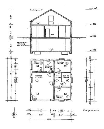
Fig. 1: Plan of testhouse
