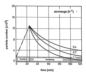
Fig. 3: Number of 1  $\mu$  m-particles after cigarette smoking with different ventilating systems
