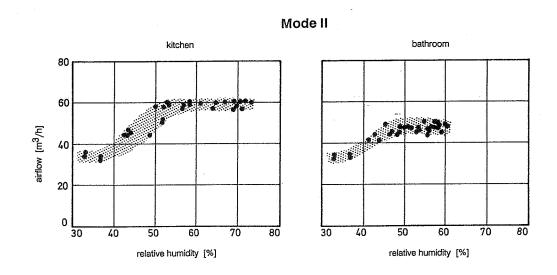
Measured values of airflow through air outlets in kitchen and bathroom for different rates of relative humidity and "mode II". (Range of regulation announced by manufacturer is from 23 % to 58 % r.h.)
