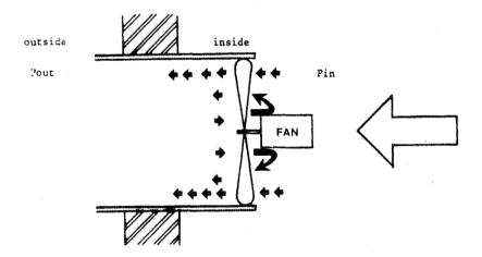
Figure 2. Back flow effect of an axial fan ( $P_{in} << P_{out}$ ).
