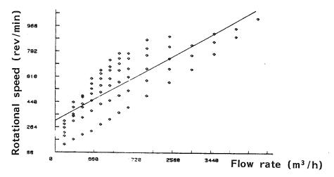
Figure 7. Linear regression analysis. Turbinemeter old design (flow rate :  $200\text{-}5000 \text{ m}^3/\text{h}$ ,  $\Delta p\text{-}120 \text{ Pa}$ ), downstream position, combined with Woods 2100 - fan.
