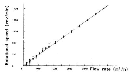
Figure 8. Linear regression analysis. 2-blade impeller prototype (flow rate :  $200-5000 \text{ m}^3/\text{h}$ ,  $\Delta p$  : 0-120Pa), upstream position, combined with Siemens 2CC2 - fan.
