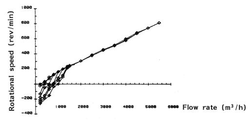
Figure 5a. Rotational speed vs. flow rate for a 2-blade impeller, downstream position.
