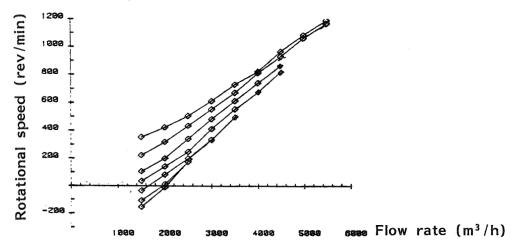
Figure 5b. Rotational speed vs. flow rate for a 2-blade impeller, upstream position.
