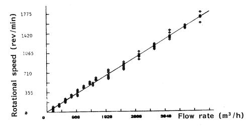
Figure 6. Linear regression analysis. 2-blade impeller prototype (flow rate :  $200\text{-}5000~\text{m}^3/\text{h}$ ,  $\Delta p$  : 0-120Pa), upstream position, combined with Woods 2100-fan.
