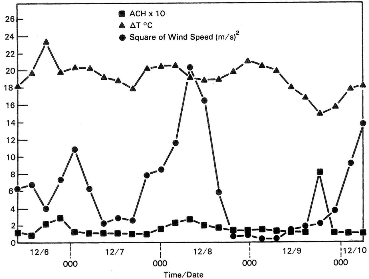
Figure 4. Measured Air Exchange Rate, Windspeed and Inside-Outside Temperature in the Bend Residence 12/5-12/10.
