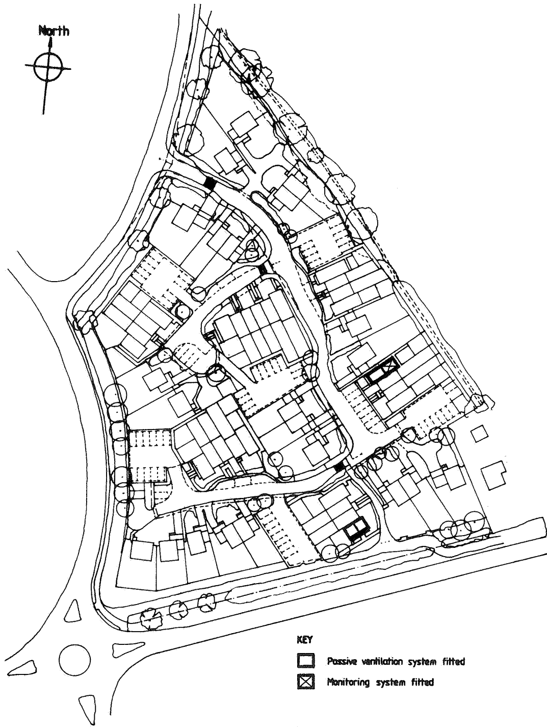
Fig 4. Site plan showing positions of houses fitted with the passive ventilation system.
