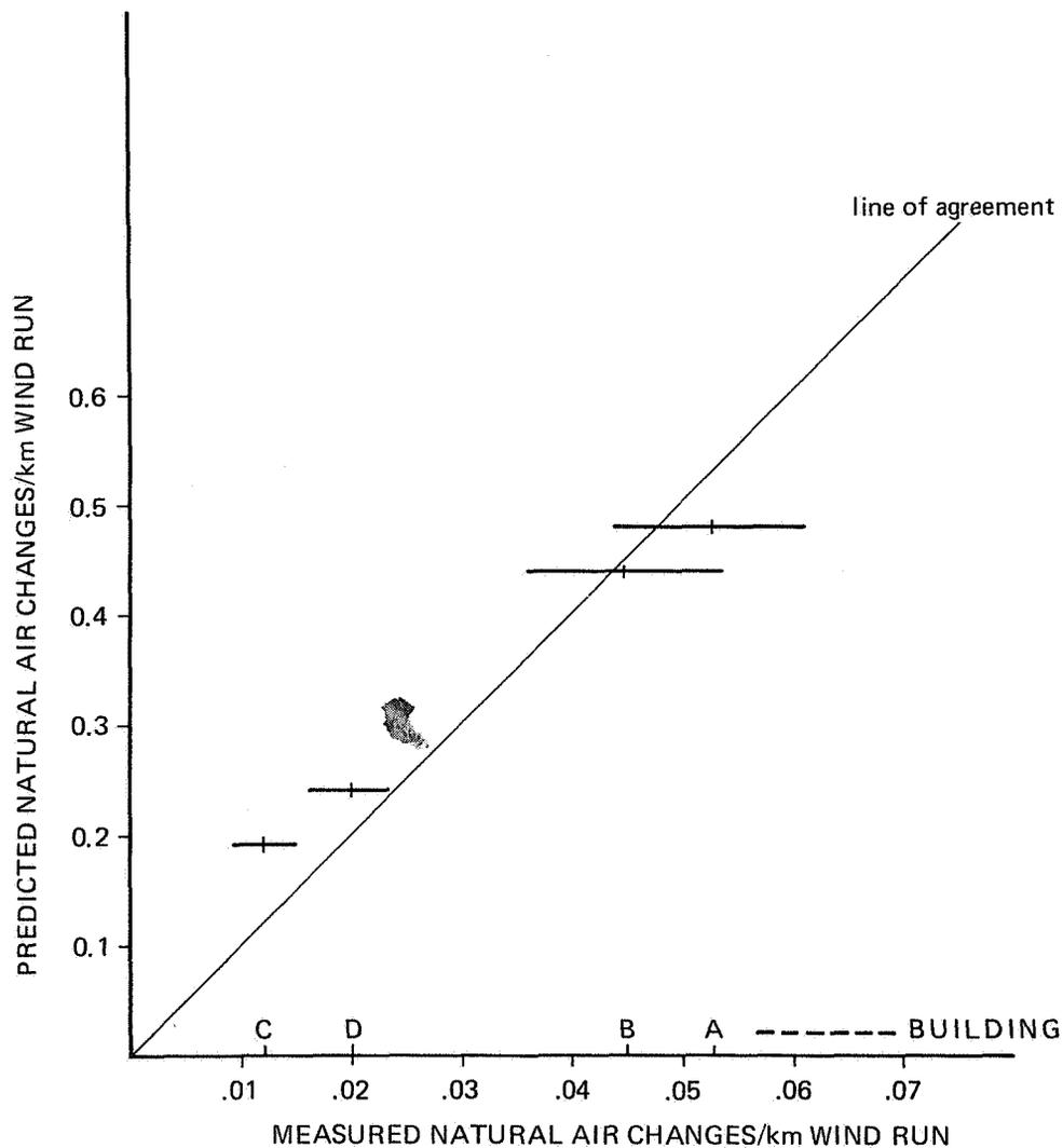
Fig 6 : CORRELATION OF INFILTRATION RATE PREDICTIONS USING SHAW MODEL WITH EXPERIMENT
